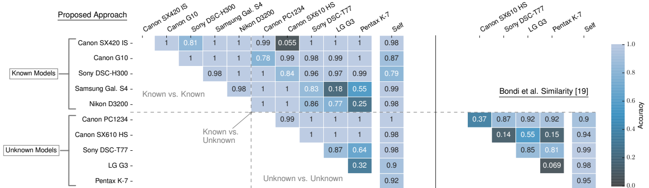
Fig. 2. Source comparison accuracy. The triangular matrices show rates of correctly detecting two patches as sourced from different camera models. The columns labeled “Self” show rates of correctly detecting two patches as sourced from the same camera model. Results of our proposed method are on the left. On the right, we compare to an approach adapted from Bondi et al. [19].
