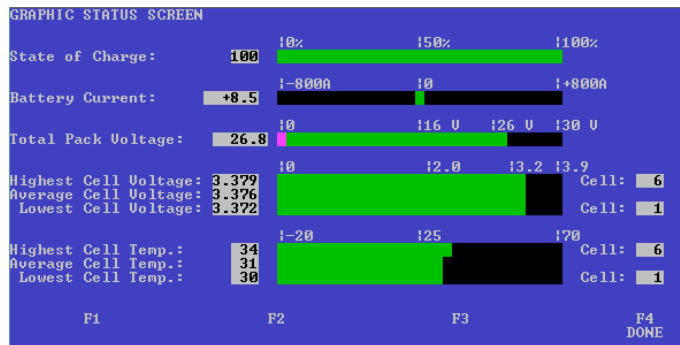
Fig. 7. Vendor-provided BMS screen for the 24 VDC, 160 Ah battery bank.
