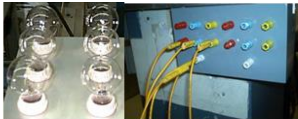
Figure 8. Resistive Loads and wye Wiring Connection
