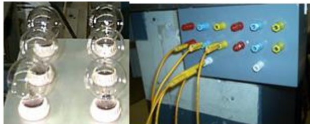
Figure 9. Resistive Loads and wye Wiring Connection
