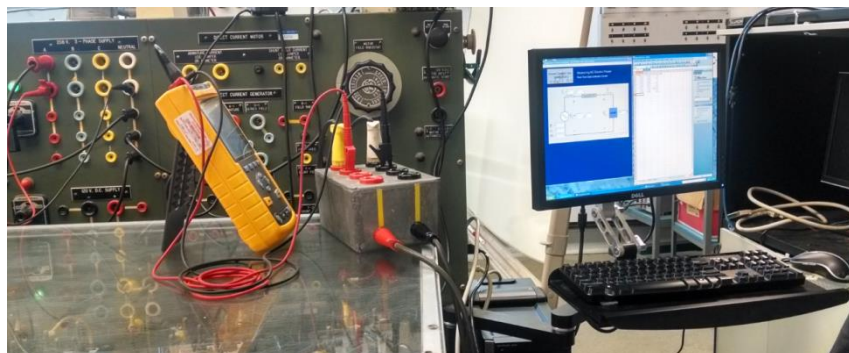
Figure 50. Inverter feed measurements
