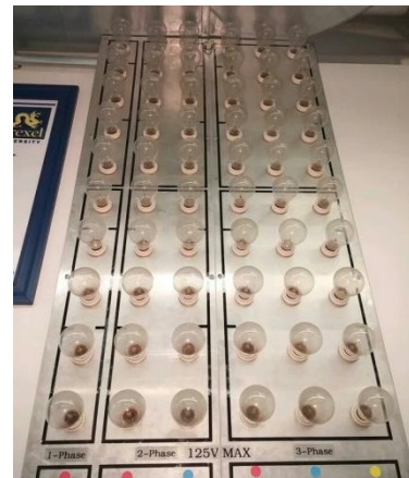
Figure 6: Load Bank Light Bulbs
