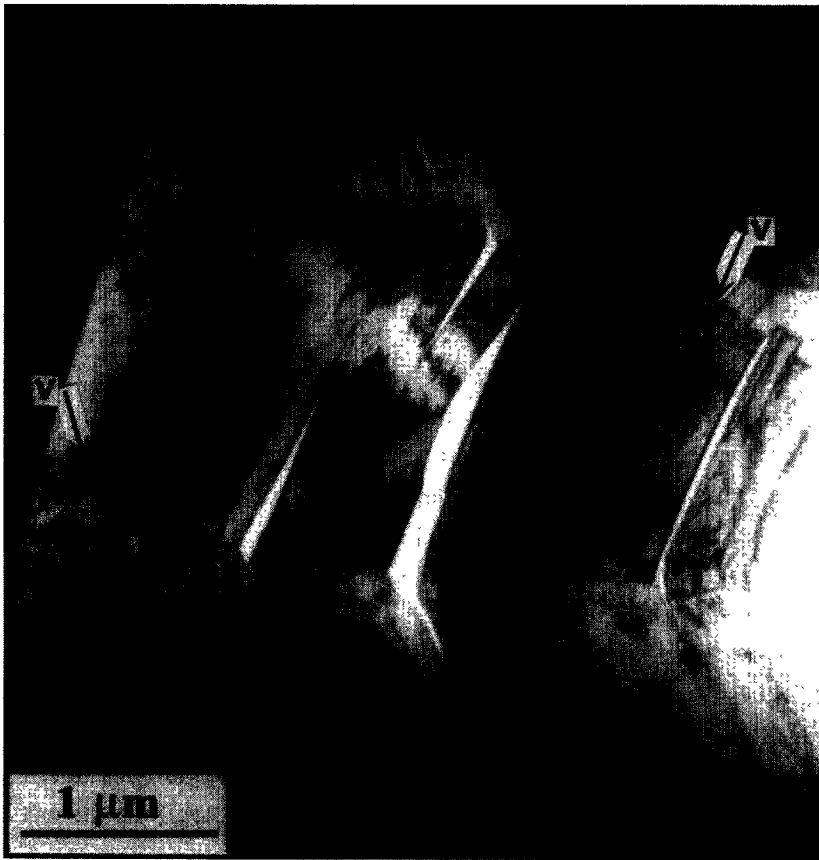
Figure 33: Bright field TEM image of a kink band with a high misorientation angle (“stove pipe”) containing delamination cracks. Separate dislocation walls, which are generally normal to the basal planes, but are inclined to the kink boundaries are denoted by V. The same areas are depicted in Fig. 29h as dark triangles.
