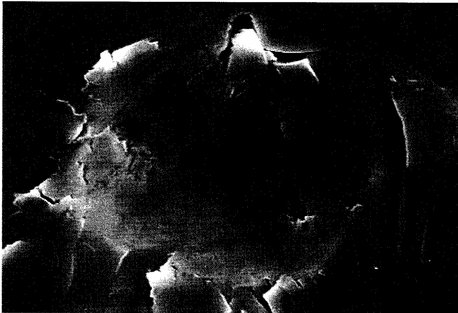
Figure 3.6: (a) Typical load-depth of penetration nanoindentation. (b) Corresponding P/\pi a^2 vs. a/R curve. (c) SEM image of an indented location by 400 N. Delamination can be seen.
