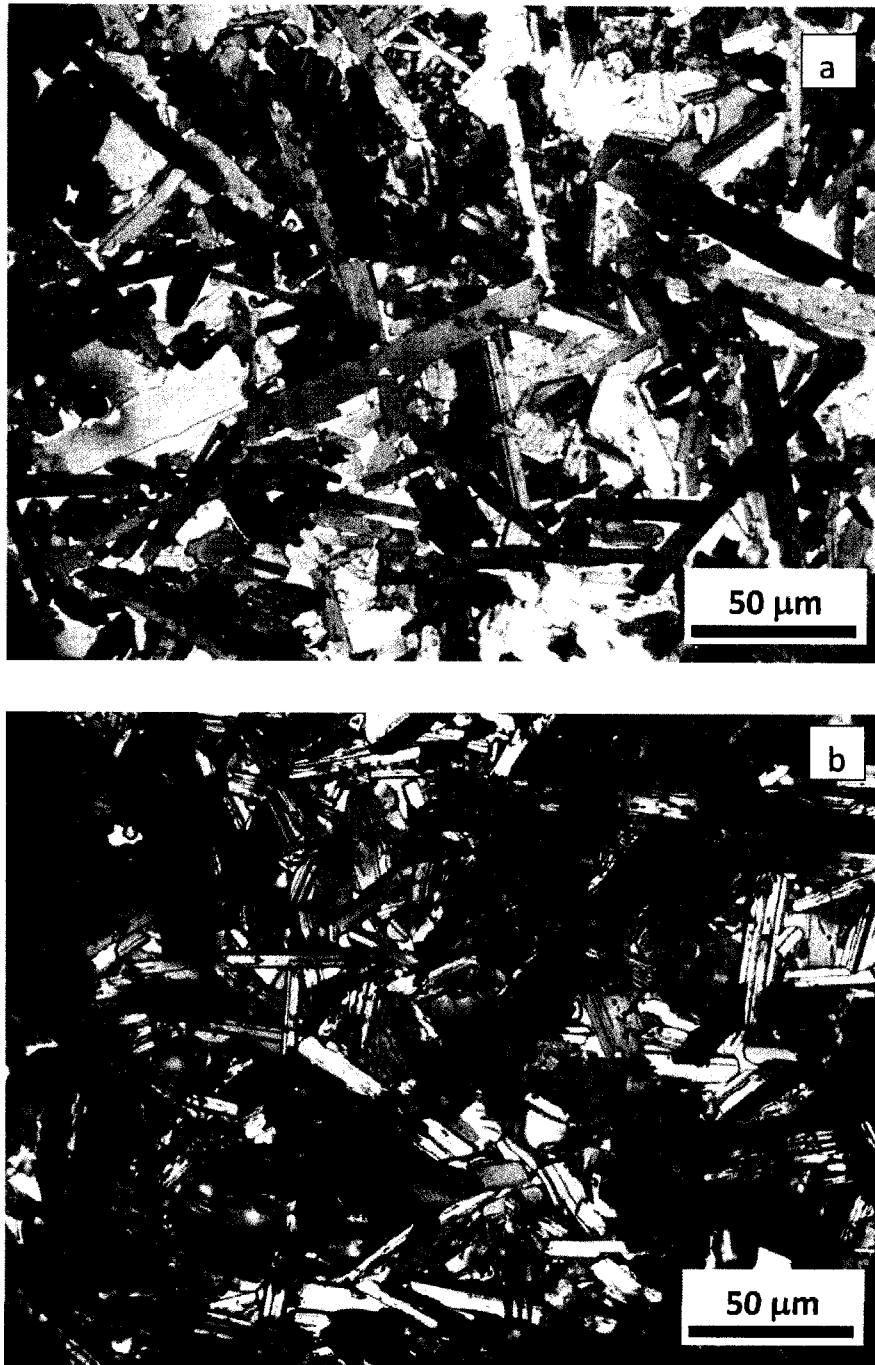
Figure 3.2: Optical micrograph of, (a) dense \text{Ti}_2\text{AlC} , (b) porous \text{Ti}_2\text{AlC} . The white areas in these micrographs are \text{TiC} .
