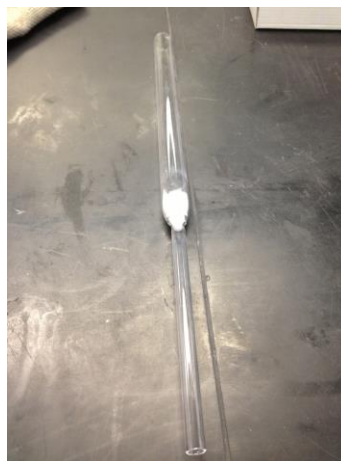
Figure 9: A quartz tube was necked down on one end while both ends were left open. The alumina crucible was inserted into the larger end and vacuum was pulled on the smaller
