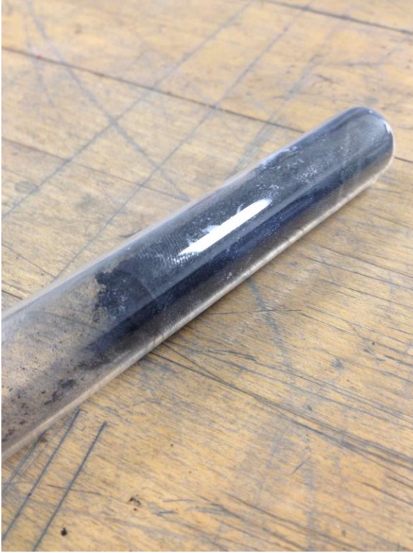
Figure 23: Crucible Sealed in Evacuated Tube This figure showed the amount of powder outside of the crucible. A much more effective method of containing the elemental mixture was required.
