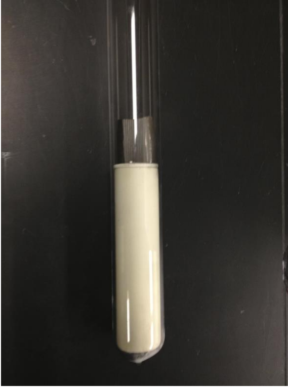
Figure 34: Sample Sealed in Evacuated Quartz Tubing
