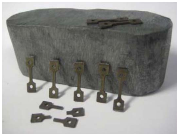
Figure 3.2 Hot pressed blank of \text{Ti}_3\text{SiC}_2 , with miniature tensile bars machined from a similar blank.
