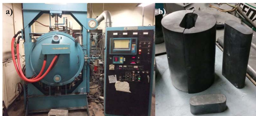
Figure 3.1. a) Uniaxial hot press, HP, used to produce MAX phase samples and, b) graphite dies used for producing MAX same.
