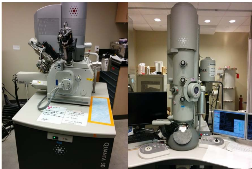
Figure 3.9 a) Quanta 3D FEG focused ion beam used to prepare TEM foils and b) FEI TF30-FEG STwin STEM used to characterize the pristine and irradiated samples.
