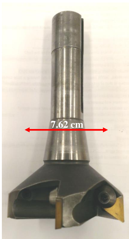
Figure 12: 7.62 cm diameter shell-inserted tungsten carbide mill
