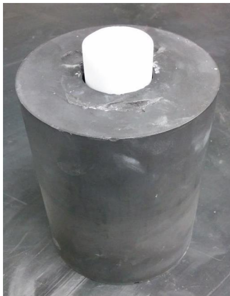
Figure 13: Picture of graphite die with a 70mm high boron nitride coated punch extending out of the die bore.
