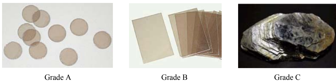
Fig. 8.2. Photographs of three different grades of mica single crystals used in herein. Grades A and B are high quality; grade C, is the most defects, as evidenced from its lack of transparency.
