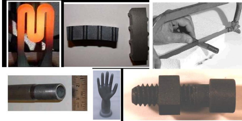
Figure 1-3: MAX Phases are superbly machinable ternary carbides and nitrides (Photos by courtesy of 3-one-2 LLC) and can be machined with ease to net-shape components.
