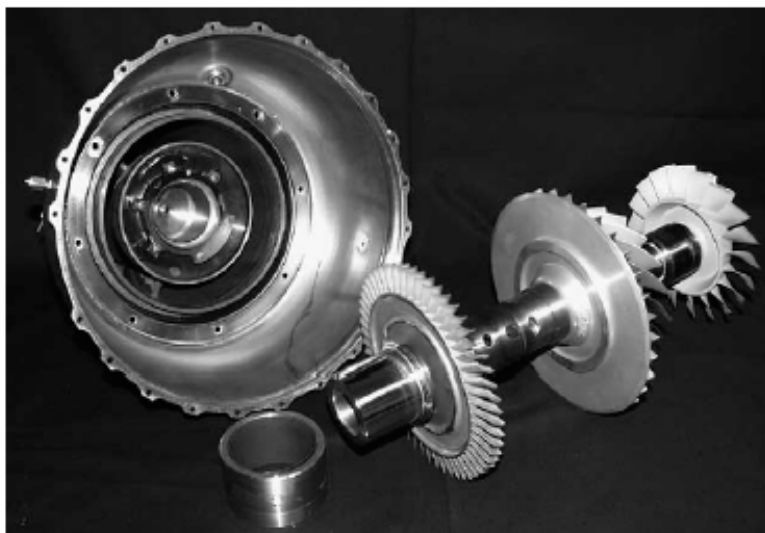
Figure 9: Oil free turbojet engine designed by Mohawk Innovative Technology, Inc., Albany, NY [Ref. 19].
