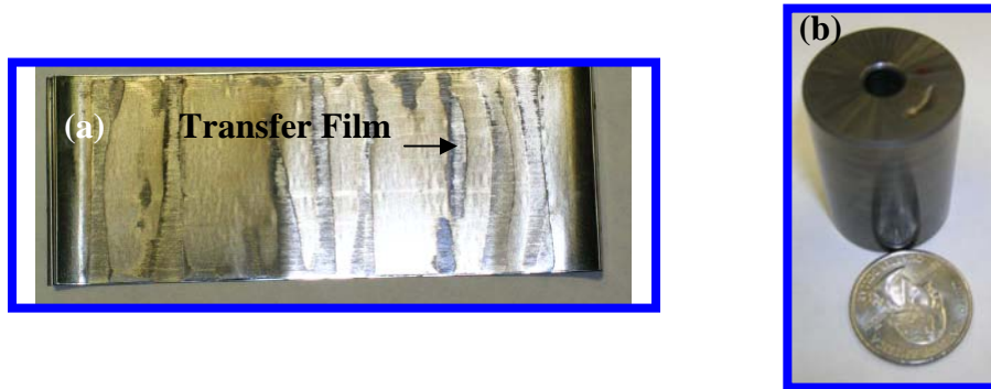
Figure 53: (a) Ni-based SA top foil, and (b) TaAgR sample, after testing in foil bearing rig at Honeywell International Facility (Torrence, CA).
