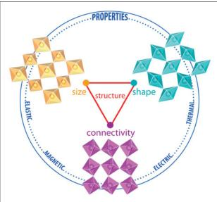
Figure 1. The interplay among different structural distortions of the octahedral units-their size, shape, and connectivitydictates the functional elastic, magnetic, electric, and thermal properties.
