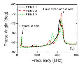
FIG. 1. (Color online) (a) An optical micrograph of array PEMS and (b) resonance spectra with detection peaks indicated.
