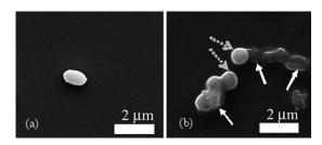
FIG. 5. SEM micrograph of PEMS sensor surface after exposure to (a) sample A  $-3.3 \times 10^3$  BA spores/ml, and (b) sample D  $-3.3 \times 10^3$  BA spores/ml with a  $3.3 \times 10^6$  cells/ml of SA and PA mixture. The solid arrows in (b) indicate BA spores which are cigar-shaped as shown in (a) while the dashed arrows indicate SA cells which are spherical.
