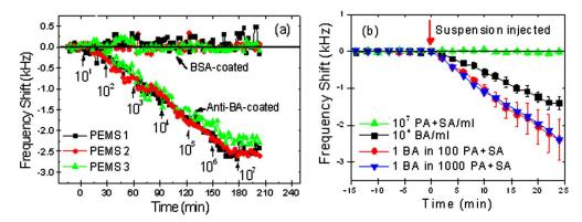
FIG. 4. (Color online) (a) Resonance frequency shift vs time of anti-BA- and BSA-coated PEMS array in BA suspensions of various concentrations, and (b) resonance frequency shift vs time of anti-BA coated PEMS array in BA suspensions in the presence of excess SA and PA cells. Arrows in (a) indicate the times of suspension injection into the flow chamber.
