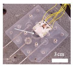
FIG. 3. (Color online) A photograph of the polycarbonate fluidics cartridge with the array PEMS mounted in the center. White arrow indication array PEMS location in the semicirculate flow chamber.
