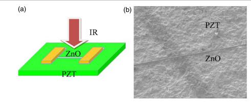
Figure 1. ZnO nanowire based on PZT transistor: (a) a schematic illustration of device configuration under IR illumination; (b) SEM image of the device showing a single ZnO NW bridging two patches of PZT.
