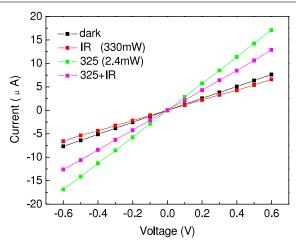
**Figure 5.** The drain current as a function of drain voltage of a ZnO–PZT transistor with an upward polarization under UV laser of 325 nm wavelength and IR illumination. The drain current can be easily modulated by tuning the powers of incident UV and IR lasers separately or simultaneously.
